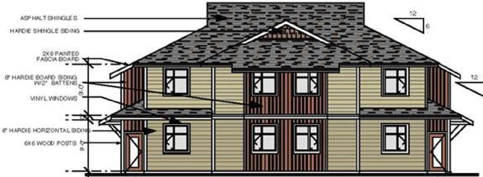
ENTRY TO UPPER UNIT ENTRY TO UPPER UNIT BLDG 4 STACKED TOWNHOUSE - FRONT ELEVATION SCALE 1/16"=1'-0"
